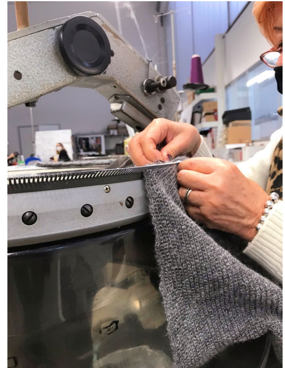
Circular Knitting Maschine used for combining knittwear pieces from our factory visit in Italy 2021.
